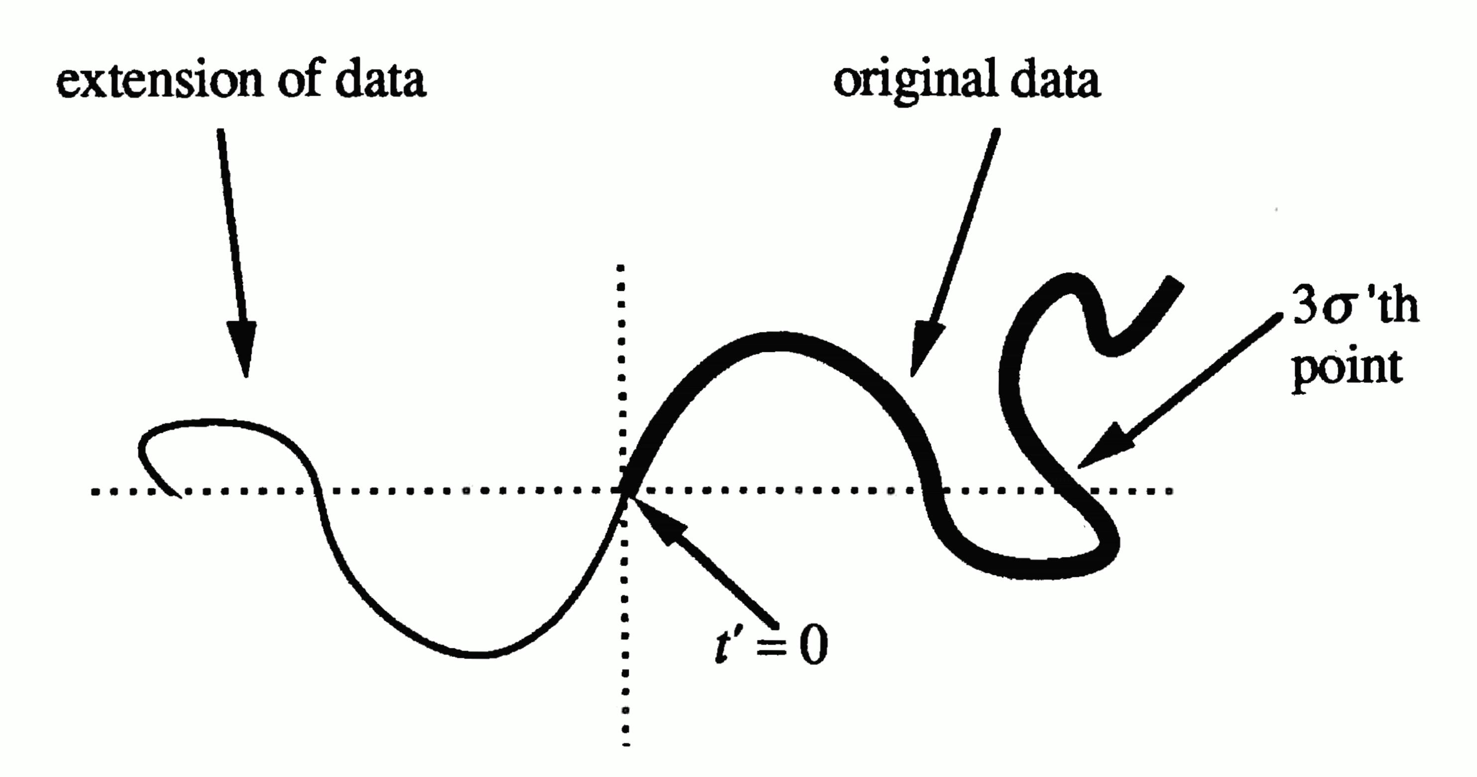
figure 4 - the curve extension ensures smoothed endpoints do not drift
