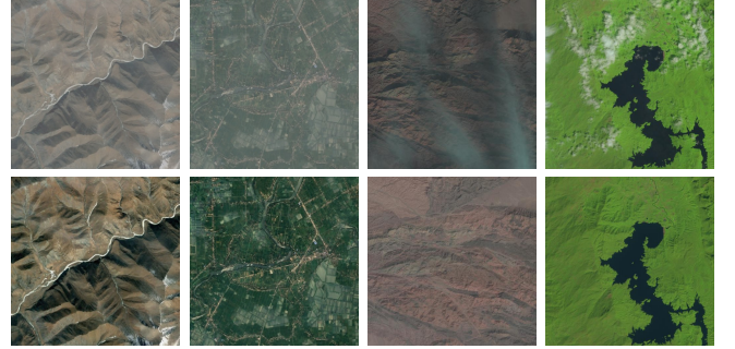
Fig. 2. Dataset samples of RICE dataset. The top row displays cloudy images, while the bottom row shows cloud-free images. The first two samples on the left are from RICE1, while the two samples on the right are from RICE2.
